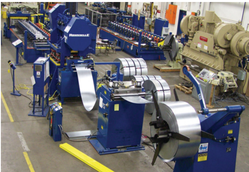
Note the length of this rollforming line, arising from the need for material loops and the use of inline processing equipment prior to the actual rollforming operation.
